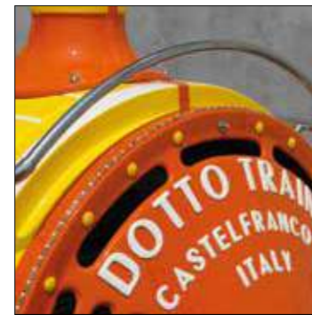
Decorative led lighting system around locomotive's front
