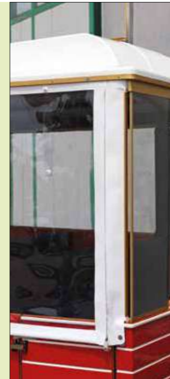
Combined closure with PVC covers and glass
