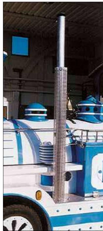
Upwards external stainless steel exhaust
