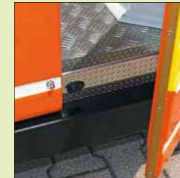
Electric door contacts (signalling any open doors)
