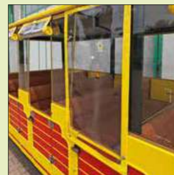
Combined closure with PVC covers and glass
